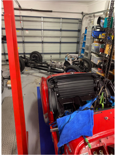
The chassis being lined up for the 'marriage'
