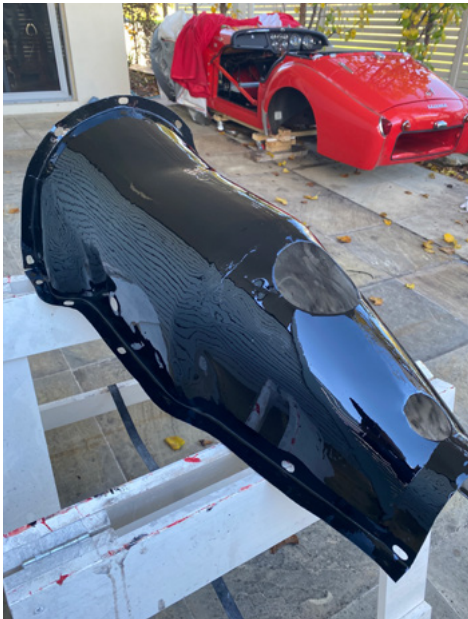
Gearbox tunnel painted
