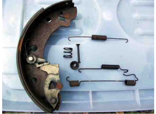
Handbrake adjusting ratchet, view of the inside of the brake shoe
