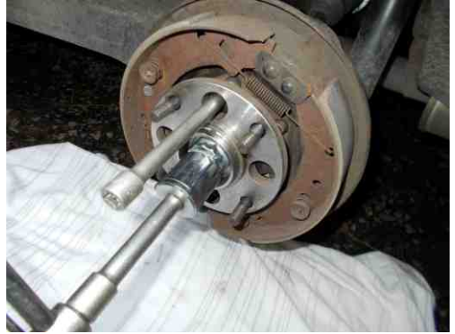
Locking the axle in place for torquing
