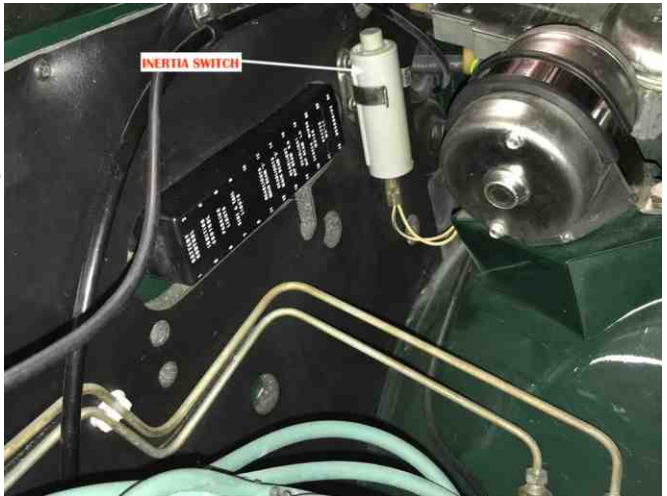
Photo 1: Location of the Inertia Switch
