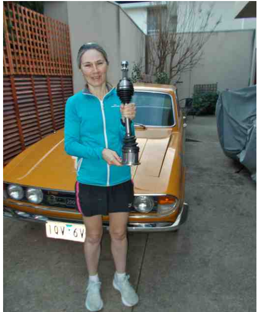
New axle, minus adaptor flange and hub, with Robyn Faithfull
