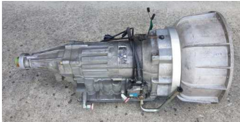
The A43DL (ex-Toyota) box, with adaptor and Stag bell housing, ready to fit into the car
