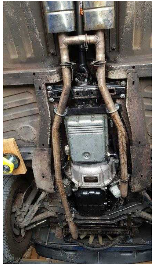
The AW box installed and ready to go. How neat is that! Hard to tell that is not the factory fitted original
