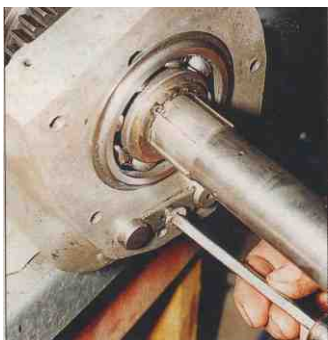
The bearing on the rear end of the mainshaft has a circlip around its perimeter outside the gearbox casing and there is a washer and a circlip on the shaft itself. The small plate, secured by a Posidrive screw, locks the layshaft and reverse gear shaft in their respective positions
