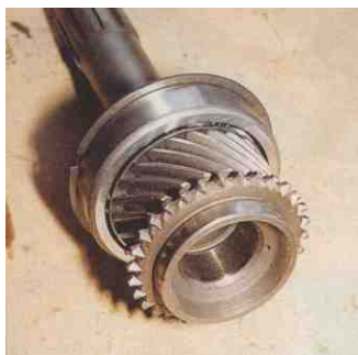
Note the oil thrower washer between the gear and the bearing on the input shaft
