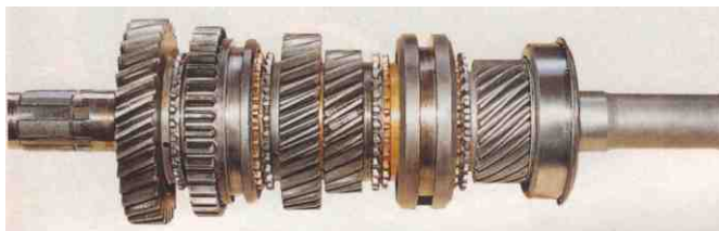
The mainshaft and input shaft assemblies: The latter with its bearing is on the right and the bearing for the rear end of the mainshaft was fitted after the shaft was placed back in the box
