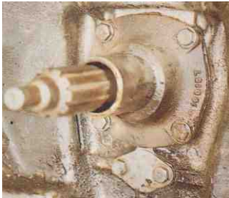
With the four bolts removed the front cover (nosepiece) was free to slide off the input shaft complete with the oil seal which it contains. The lower cover came off later to release the layshaft
