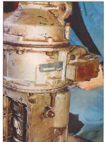
Note the extra long stud at the overdrive/gearbox flanges (there is one on the other side too) to allow the internal spring pressure to be released gradually
