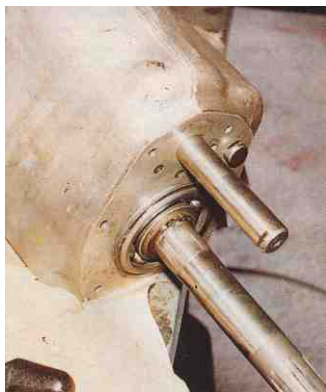
With the gearbox upside down and the mainshaft and input shaft assemblies already in position, the layshaft cluster should drop into the correct position for its shaft to be inserted
