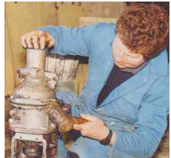
Having loosened all the nuts Chris tapped the casing with a mallet to break the seal. Overdrive is the 'A' type
