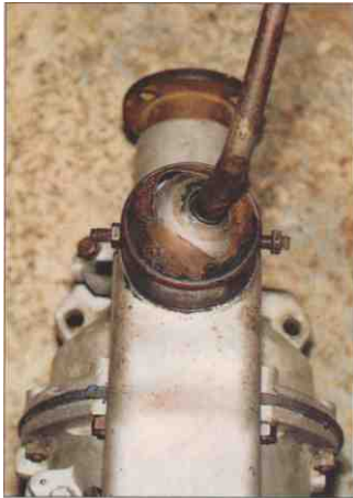
The adjusting screws and locknuts which are used to take up excess movement in the gearlever can be seen on each side of the gearlever housing
