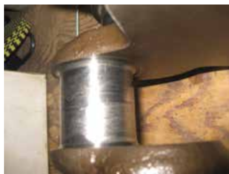
Scoring on the crank journal and bearing shells was responsible for the knocking noise from the #5 big end
