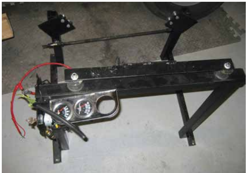
Tony added coolant temperature and oil pressure gauges to the rig
