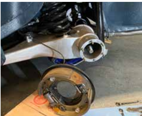
The hub and brake backplate were removed, the backplate was placed on a box to support it
