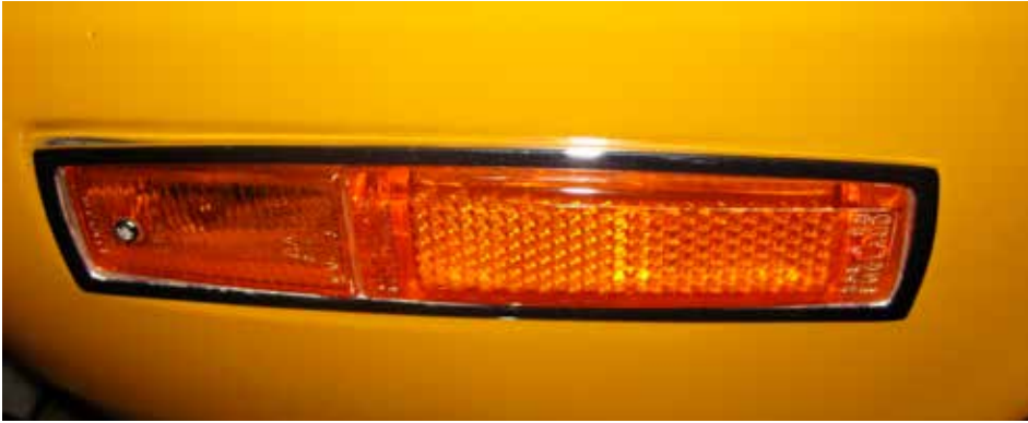
The earlier style side marker lenses were attached with one screw
