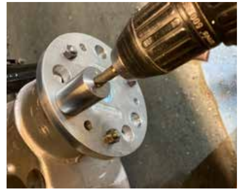
The hole was drilled out bigger using the special drill sized insert
