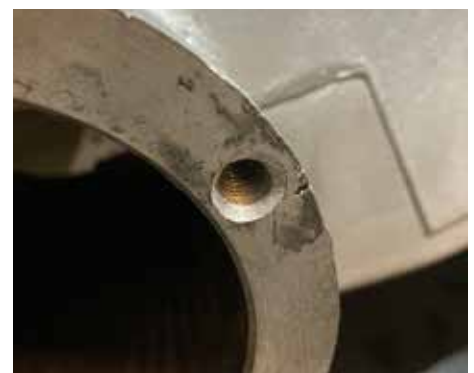
The new threads were countersunk a little to ensure that any shoulder left does not interfere with the hub/backplate
