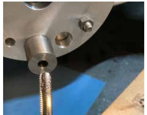
Swarf prevents the tap bottoming so it was blown out with air and the tap ran in again
