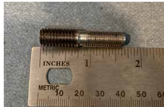
The Stud had the 3/8 UNC thread extended down the shoulder and the 3/8" section was shortened down to just under 3/4" (18mm)
