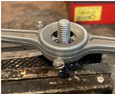
Cutting the 3/8" UNC thread into the shoulder. The fine end was locked with 2 good quality grade 8 nuts and held in the vice
