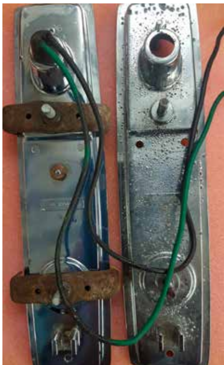
The base of the units look similar, but some holes have been blanked off
