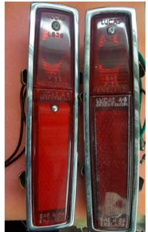
The later type (left) were held in place with two screws
