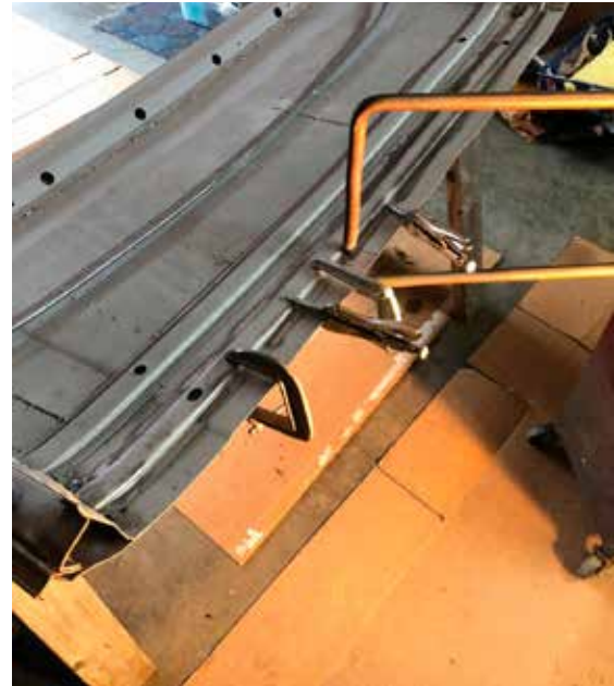
Extra support "beam" taken from front of hardtop so that bow gusset can hold up against it with headliner
