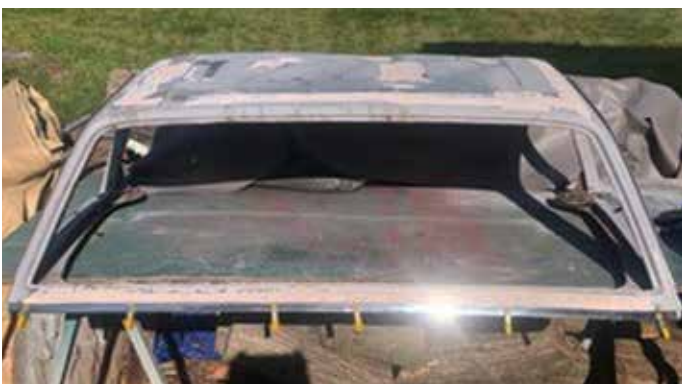
There were no guide holes remaining to drill and pre-fit the rivets for the stainless steel trim strips
