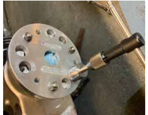
Then it was tapped out using the tap sized insert
