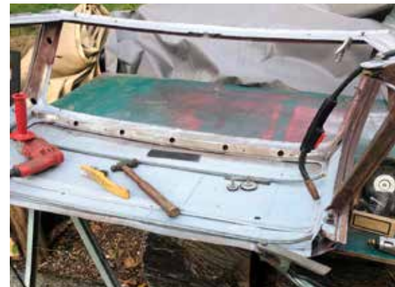
Bow gusset to hold headliner retained
