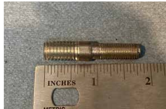
The Triumph Motorcycle cylinder stud as bought. There is a short section of 3/8" shoulder that needs to be eliminated
