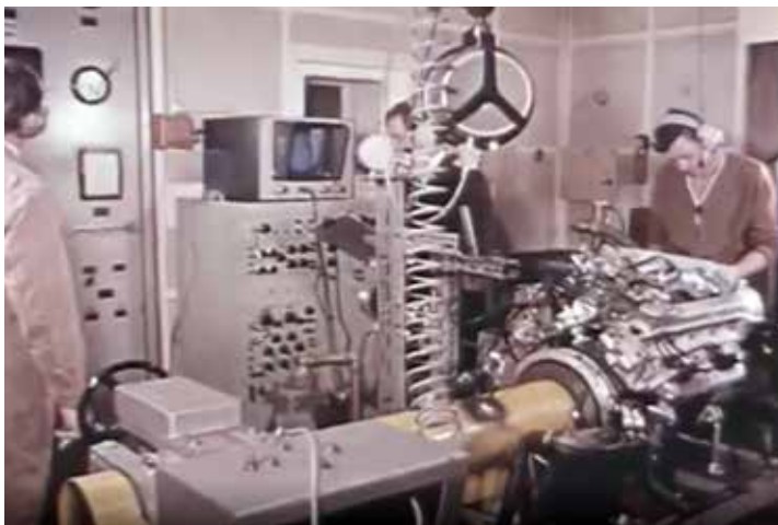
A USA spec engine being tested on one of the dynamometers at Canley. Image: from 'This is Triumph', a promotional film from 1971/72
